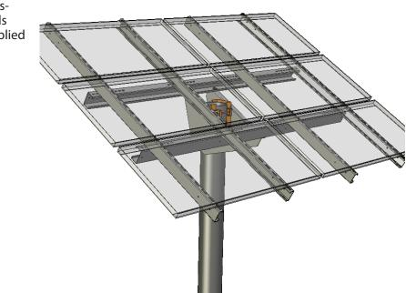
2. Adjust the tilt of the panel, then tighten the tilt plate nuts to 12 ft-lbs.
